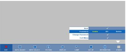
**b** Enabling the Password function will pop up a character screen, key in a 4-digit number from the screen and press  $\overline{\mathbb{A}}$ .
