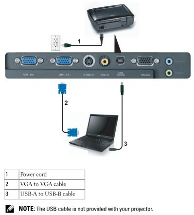
**NOTE:** The USB cable must be connected if you want to use the Page Up and Page Down features on the remote control.
