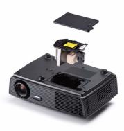
**9** Reset the lamp usage time by selecting "Yes" for **Lamp Reset** in the OSD **Lamp** tab (see Lamp menu on page 34). When a new lamp module has been changed, the projector will automatically detect and reset the lamp hours.
